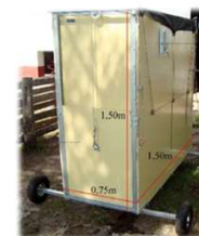
Isolation Box Test (Blache & Ferguson, 2005)
