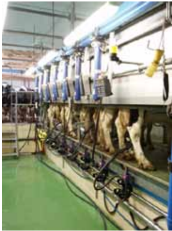
Delaval Milking Parlour with milk meters
