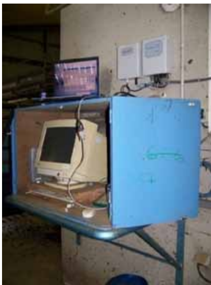
The weighing system and the electronic tag reader are connected up to a computer. The reader makes a sound once it has detected an electronic tag on an animal. The animal's weight and number are entered automatically.
