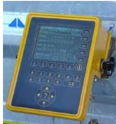
Operates the doors once the number of the animal sent by the reader has been checked
