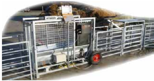
EIDTrace reading-weighing device (Farms, the Lot region).
