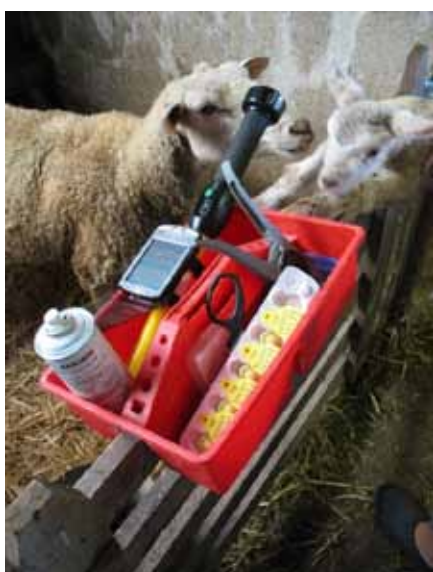
Stick type mobile reader connected to a PDA running a cattle management application via a Bluetooth® connection. Platform carries the PDA fixed to the reader.
