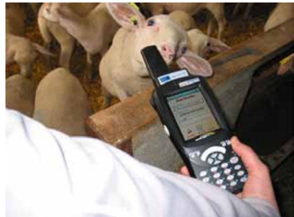
Once a number has been read electronically, the information associated with this number can be read using the cattle management software installed on the all-in-one reader.
