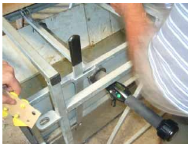
Collar fixed to a chute so a stick type mobile reader can be used in a fixed configuration (cattle crush).
