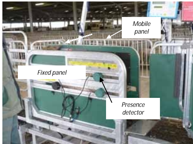
Racewell device [animals blocked in at the side (vice)] (Parthenay market, Deux-Sèvres).
