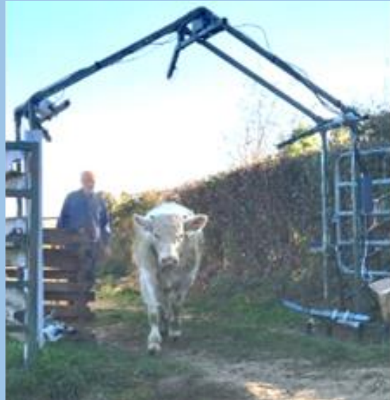
A movable gantry Embedding 10 RGB-D sensors
