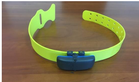
Figure 3. GPS device attached on designated collar.
